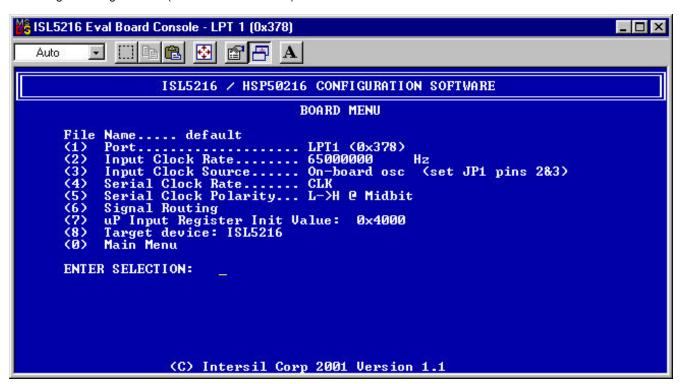
Port and Input Clock Source options apply only to the evaluation board. These settings may be ignored if an evaluation board will not be connected. The software can be used to generate register files even without an evaluation board. In this case, use main menu option 10 ("compute
