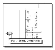
For 220/240 volts AC, the supply is connected to the lower 0 volt terminal and the upper 110 volt terminal and a shorting wire connected between the middle 0 and 110 volt terminals of the AC Mains Supply, i.e. series connection of the transformer.
