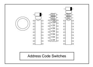
If more than one system is to be used in close proximity, each system can be set to a unique code such that one transmitter will not operate the other control. This facility can also be used for low level security purposes.
