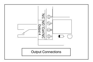
Individual relay outputs can be configured to be Momentary or Latching. The default function, from the factory, is set to Momentary.
