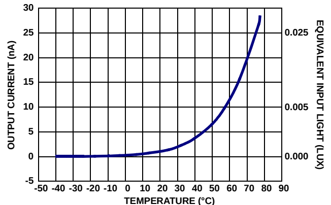
FIGURE 11. OUTPUT CURRENT vs TEMPERATURE AT 0 LUX
