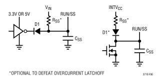
Figure 6. RUN/SS Pin Interfacing
