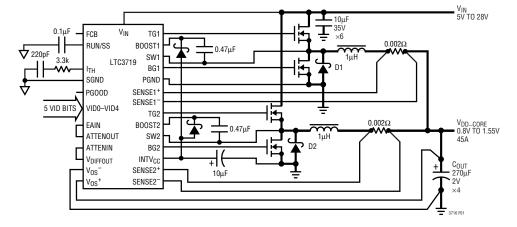
Figure 1. High Current Dual Phase Step-Down Converter
