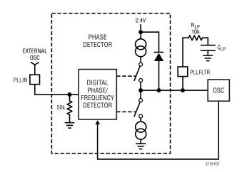
Figure 7. Phase-Locked Loop Block Diagram
