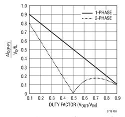
Figure 3. Normalized Output Ripple Current vs Duty Factor  $[l_{RMS}\approx 0.3~(\Delta l_{O(P-P)})]$
