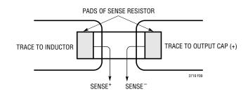
Figure 9. Proper Current Sense Connections
