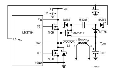
Figure 5b. Capacitive Charge Pump for EXTV<sub>CC</sub>
