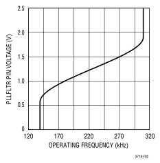
Figure 2. Operating Frequency vs V<sub>PLLFLTR</sub>
