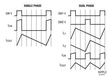
Figure 11. Single and 2-Phase Current Waveforms
