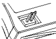
Figure 8: Master Setting for Vertical iDiskOnChip 44-Pin Connector
