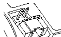
Figure 9: Master Setting for Vertical iDiskOnChip 40-Pin Connector
