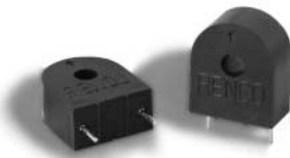
These encapsulated Current Sensing coils are designed for PC board mounting and are used as a nonintrusive method of controlling, monitoring or measuring AC currents. The sensors are non-contact devices having no DC power loss resulting in no heating problems. High quality toroids are used in order to obtain optimum performance over the designated current and frequency range.
