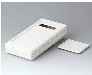
A9074207 DATEC-MOBIL-BOX M, Vers. II ABS (UL 94 HB) off-white RAL 9002 7.68"x3.98"x1.73" IP 65 opt.
