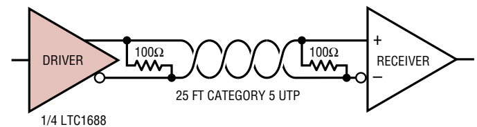
Figure 12. 100Mbps Differential Data Connection
