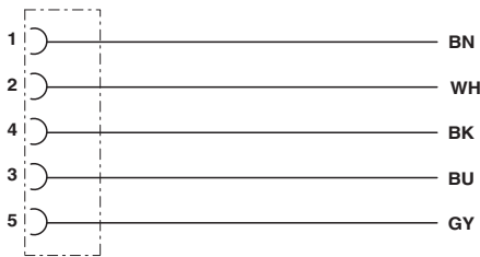
Contact assignment of the M12 socket
