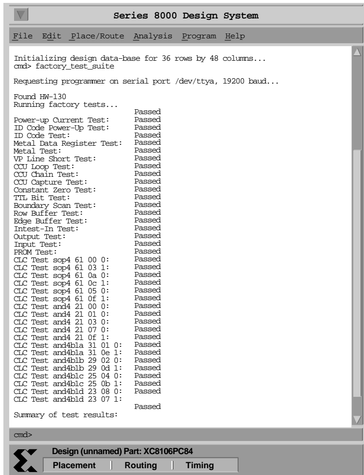
Figure 17: Series 8000 Software Testing a Device in an HW-130
