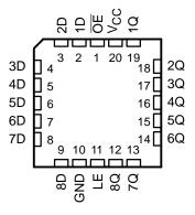
OE does not affect the internal operations of the latches. Old data can be retained or new data can be entered while the outputs are in the high-impedance state.
