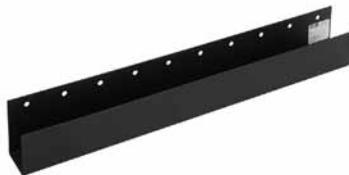
For routing cable front-to-back in a server or data cabinet. Mounts to side or top of 1- or 3-row grid strap. Can also mount directly to mounting channels with APSM6CN Mounting Kit. Multiple units can be used together. 16 gauge steel with RAL 9005 black polyester powder paint finish.
