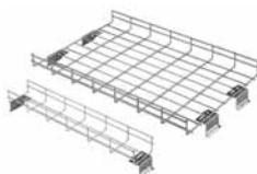
The Basket Tray mounts horizontally left-to-right in the PROLINE® frame. It can be installed either at the bottom of the frame or to the mounting strut and can provide an internal cable runway in a row of cabinets. Large 51 x 102-mm (2 x 4-in.) mesh allows cable installers to route cables in or out at any point. Made of plated high strength steel wire. Includes mounting hardware.
