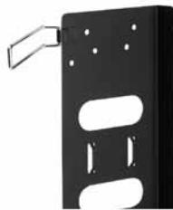
For routing and bundling cable inside cabinets. Stack two units for full vertical runway on 1800-mm or taller enclosures. Wireform gate hinges open to ease wire routing. Mounts to grid strap or frame in front of rack angles. Narrow profile does not interfere with 19-in. equipment in 600-mm wide enclosures. 16 gauge steel with RAL 9005 black polyester powder paint finish.
