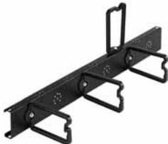
Manages cable routed between front and back of cabinet. Can be used with optional Universal D-Ring Brackets or Transition Brackets for increased flexibility in managing cables. Mounts to PROLINE frame. Secures cable with D-Rings that snap open and closed for secure routing with easy access for wiring changes. D-Rings can be oriented for vertical, front-to-back or side-to-side cable management. RAL 9005 black polyester paint finish. Includes D-Rings and mounting hardware.
