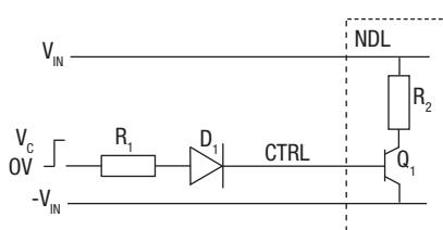
D<sub>1</sub> (e.g. 1N4001) is required to provide high impedance when the signal is low. From the NDL specification, the drive current to operate this function is recommended to be 10mA, and hence the value of R<sub>1</sub> can be derived as follows:
