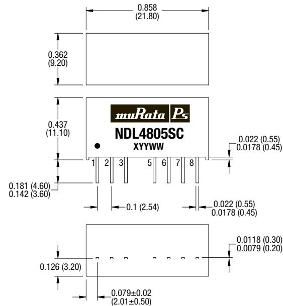
All dimensions in inches  $\pm 0.01$  (mm  $\pm 0.25$ mm). All pins on a 0.1 (2.54) pitch and within  $\pm 0.01$  (0.25) of true position.
