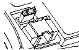
Figure 7: Slave Setting for Vertical iDiskOnChip 40-Pin Connector
