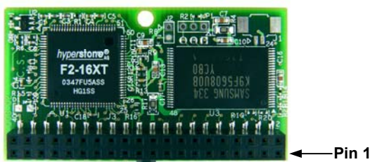
Figure 4: iDiskOnChip Horizontal Version 40 pin, Right-Oriented
