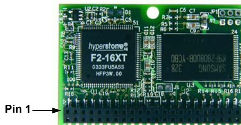
Figure 5: iDiskOnChip Horizontal Version 44 pin, Left-Oriented
