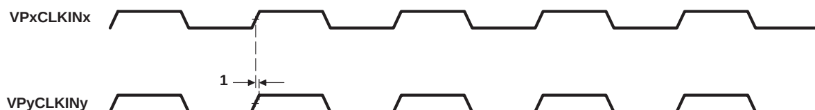
Figure 4–61. Video Port Dual-Display Sync Timing
