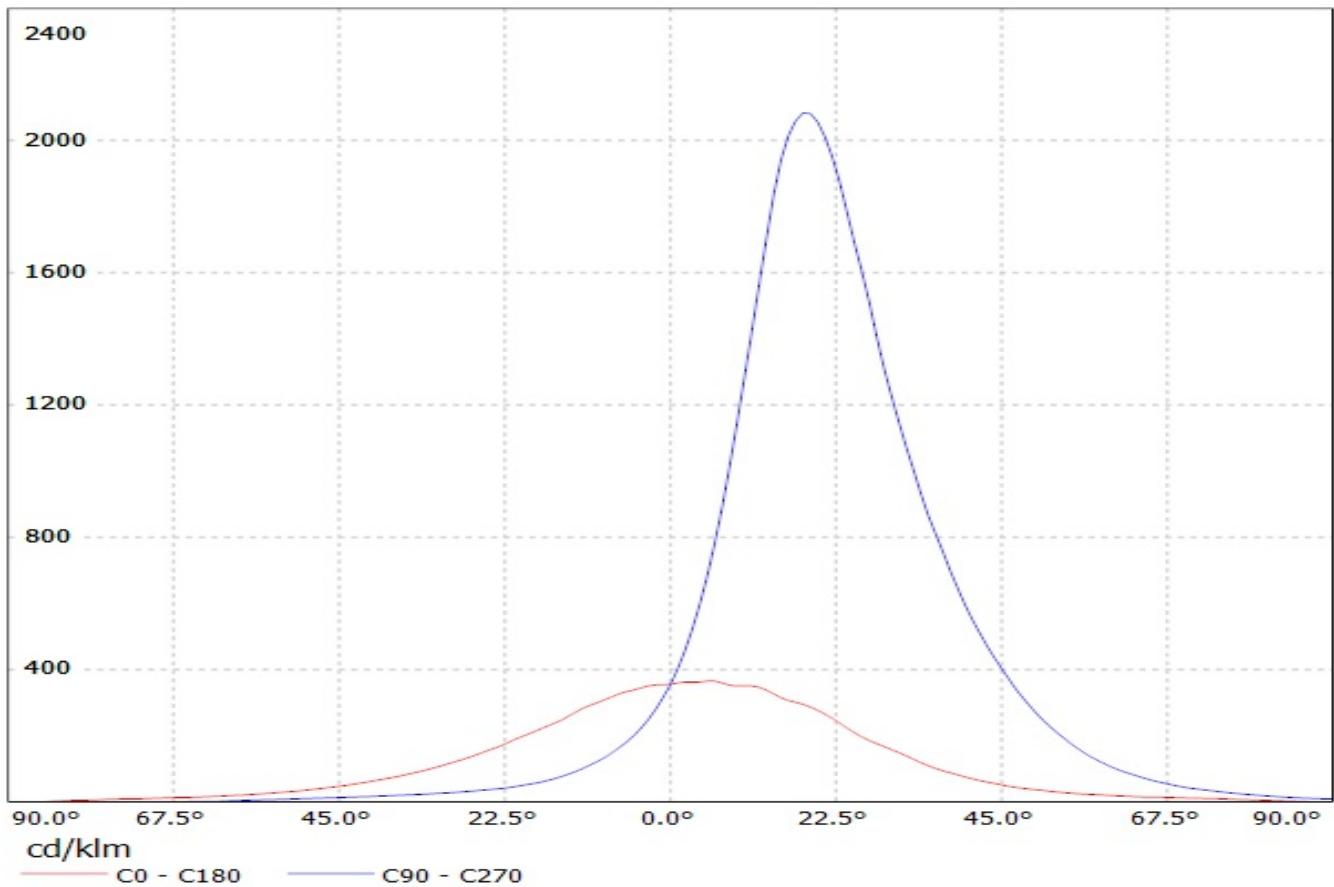
Luminaire: Ledil Oy FCA13329\_BILLIE-A (Cree XB-D 90lm @ 250mA) Efficiency=85%
