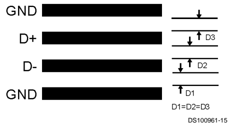
FIGURE 6. Recommended Diode Trace Layout
