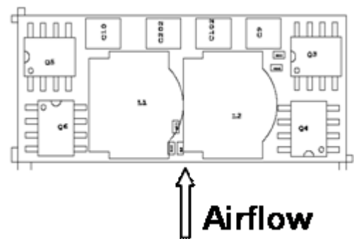
Figure 55. Airflow direction for thermal testing.
