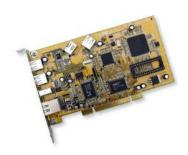
How many legacy PCs become useless simply because they lack up-to-date I/O connectivity? Sometimes all it takes to bring new life to an old PC is to add USB 2.0, Firewire or Ethernet connectivity. This is easily accomplished with a PCI Combo Card. A single addin card can have several I/O devices; but
