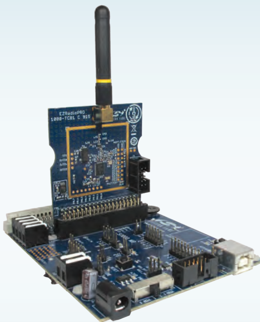
Si1000 TARGET BOARD WITH EZRadio® TEST CARD
