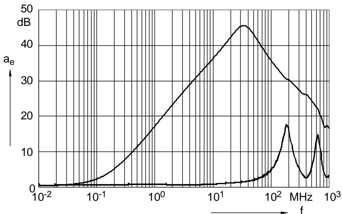
**Insertion loss  $\alpha_e$**  ( typical values at  $Z = 50\Omega$ )
