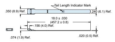
The 600-090 Extended Length Standard Band is precision constructed of 300 Series SST/Passivate, and designed for use with the 600-058 Hand Banding Tool or the 600-067 Pneumatic Banding Tool. Double-wrapped bands will accommodate diameters up to approximately 2.5 inches (63.5). Bands may be ordered flat (600-090), or precoiled (600-090-1). Bands come bagged and tagged in quantities from 1 to 100.
