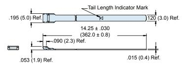
The 600-083 Extended Length Micro-Band is precision constructed of 300 Series SST/Passivate, and designed for use with the 600-061 Hand Banding Tool or the 600-068 Pneumatic Banding Tool. Double-wrapped bands will accommodate diameters up to approximately 1.88 inches (47.8). Bands may be ordered flat (600-083), or precoiled (600-083-1). Bands come bagged and tagged in quantities from 1 to 100.
