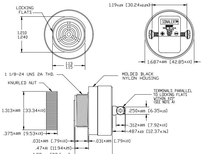
NOTE A: TERMINALS-.032 BRASS TIN PLATED, TAPPED FOR #6-32 SCREW. TWO #6-32 NICKEL PLATED BRASS SCREWS INCLUDED. WILL ACCEPT 1/4" QUICK CONNECT.
