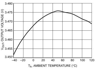
Figure 3. Output Voltage versus Temperature
