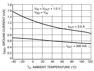
Figure 6. Ground Current versus Temperature
