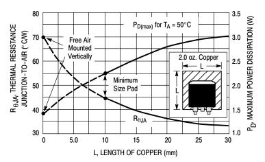
Figure 11. 3-Pin and 5-Pin D<sup>2</sup>PAK Thermal Resistance and Maximum Power Dissipation versus P.C.B. Copper Length
