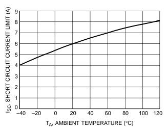
Figure 4. Short Circuit Current Limit versus **Temperature**
