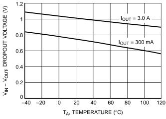
Figure 5. Dropout Voltage versus Temperature
