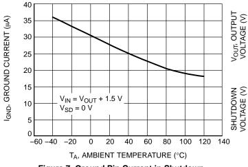
Figure 7. Ground Pin Current in Shutdown **Mode versus Temperature**
