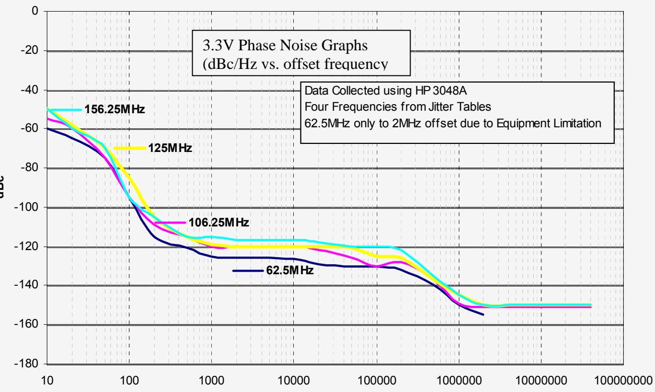
Jitter is frequency dependent. Below are typical values at select frequencies.
