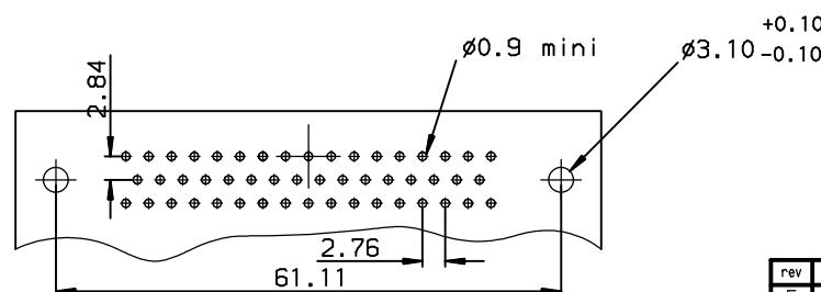
Dimensions are in millimeters
