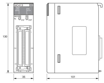
Note: The above diagram is for the CS1W-NC413.
