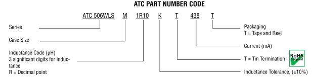
The above part number refers to a 506WLS Series, Case Size M, 1.10 µH inductor, K tolerance (±10%, typ.), with Tin Termination (T), 438 mA, tape and reel packaging.
