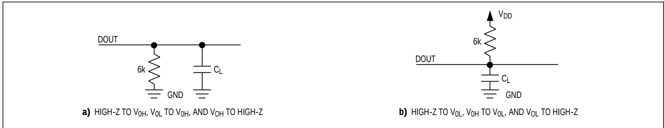
Figure 1. Load Circuits for Enable and Disable Time
