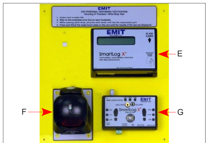
Figure 3. SmartLog X 3 ™ features and components (Items 50734, 50735)
