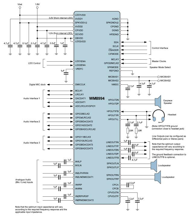
Note that input capacitors are not required for connection to Digital Microphone (DMIC) components.
