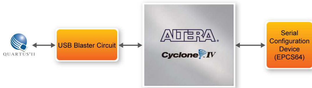
Figure 3-1 Programming a serial configuration device with serial flash loader solution
