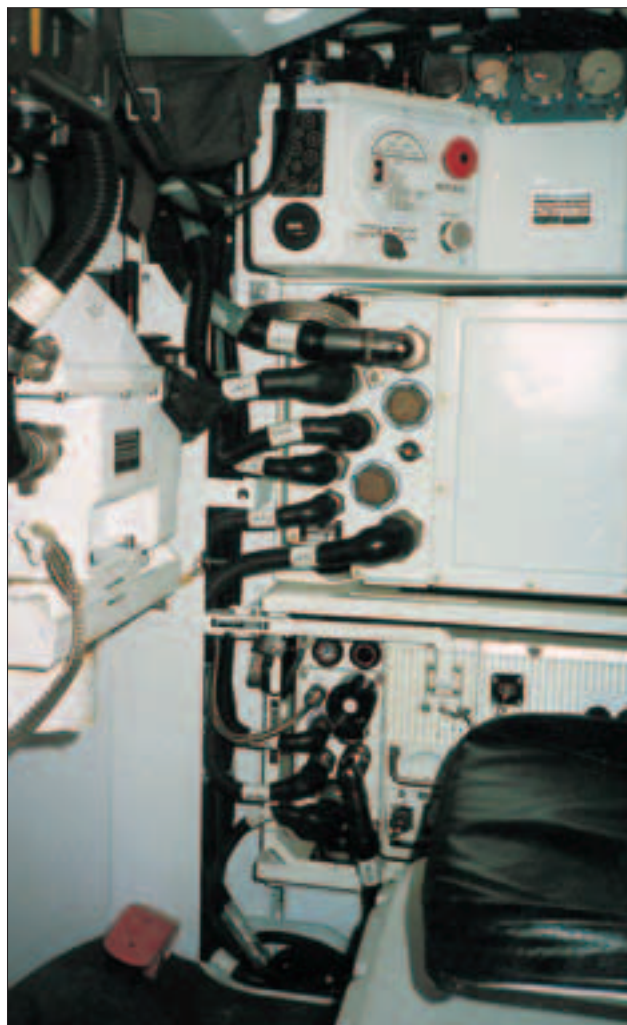
Space saving right-angle shapes used here in a military application.
