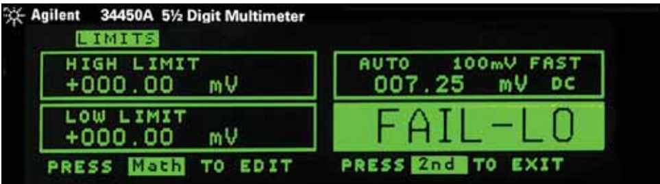
Figure 5. The display of 34450A in limit operation.
