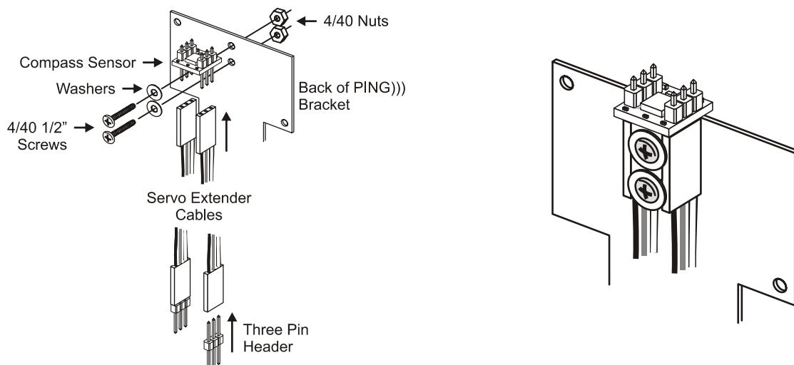
**Step 1:** Mount the HM55B Compass Module on the back side of the PING))) Mounting Bracket using (2) 4/40 1/2" screws, (2) 4/40 nuts and (2) 10" servo extension cables.
