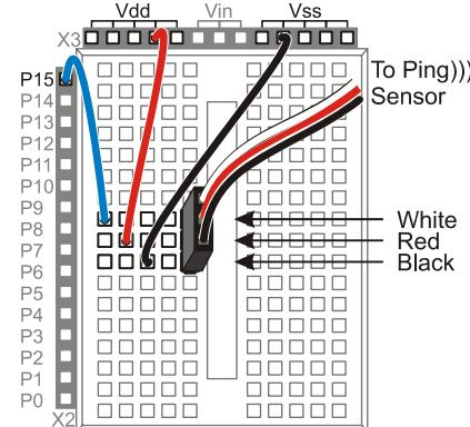
The PING))) sensor requires a 5 VDC power supply. To make the connections directly from the breadboard:
