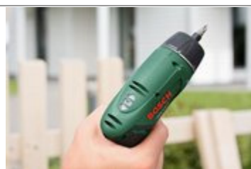
Forward/reverse indicator, battery charge level indicator and torque setting
