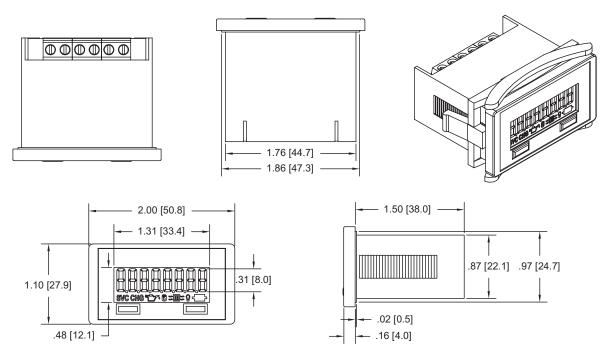
Panel Cutout: 1.79" [45.5mm] x 0.89" [22.6mm] Recommended Panel Thickness: 0.125" [3.1mm]
