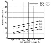
5-(2). Coil temperature rise Tested sample: TX2-48V, 6 pcs. Point measured: Inside the coil
