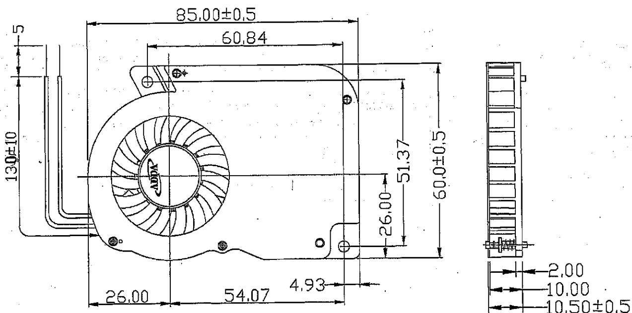
LEAD WIRES : UL 1571, AWG28, L = 130.+- 10 MM
