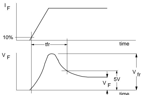
Fig.1. Definition of  $V_{fr}$  and  $t_{fr}$
