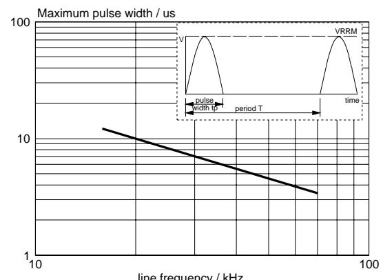
Fig.4. Maximum allowable pulse width  $t_p$  versus line frequency; Basic horizontal deflection circuit.
