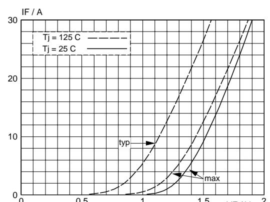
Fig.5. BY329-1500 Typical and maximum forward characteristic  $I_F = f(V_F)$ ; parameter  $T_j$
