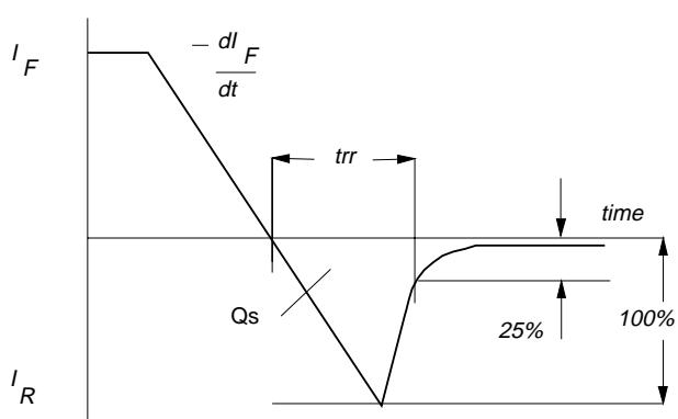
Fig.2. Definition of  $t_{rr}$  and  $Q_s$
