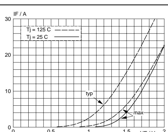
Fig.6. BY329-1500S Typical and maximum forward characteristic  $I_F = f(V_F)$ ; parameter  $T_j$
