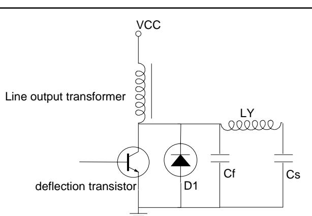
Fig.3. Basic horizontal deflection circuit.
