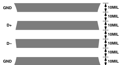
Figure 6. Arrangement of Signal Tracks
