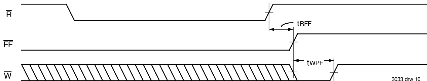
Figure 8. Minimum Timing for a Full Flag Coincident Write Pulse
