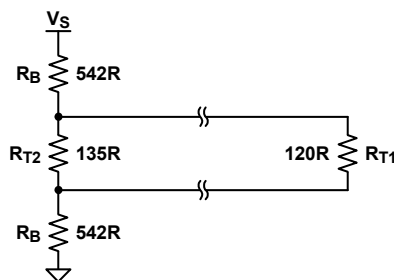
Figure 8. Single Fail-Safe Biasing for Short Data Links
