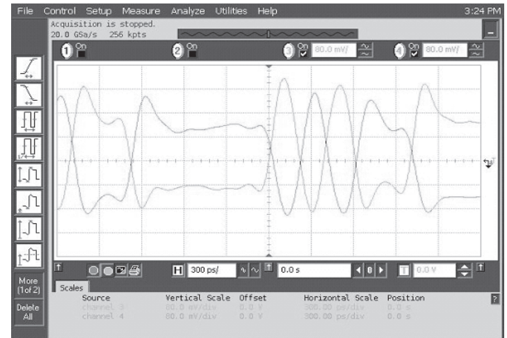
Data Waveforms, 3.0Gbps (left) & 6.0Gbps (right)
