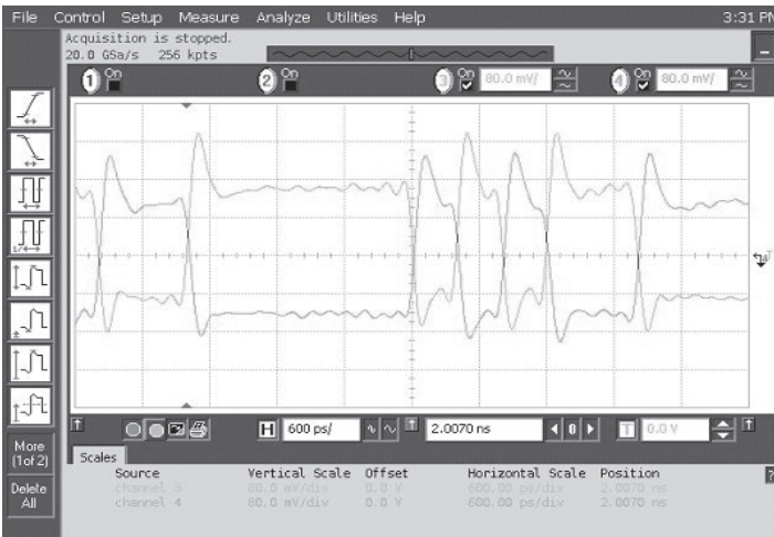
Data Waveforms, 3.0Gbps (left) & 6.0Gbps (right)
