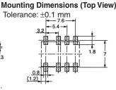
**Note 1:** Each value has a tolerance of  $\pm 0.3$  mm. Note 2: The coplanarity of the terminals is 0.1 mm max.
