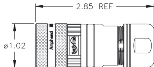
Plug kit straight, threaded; 7.5-11.0mm cord grip
