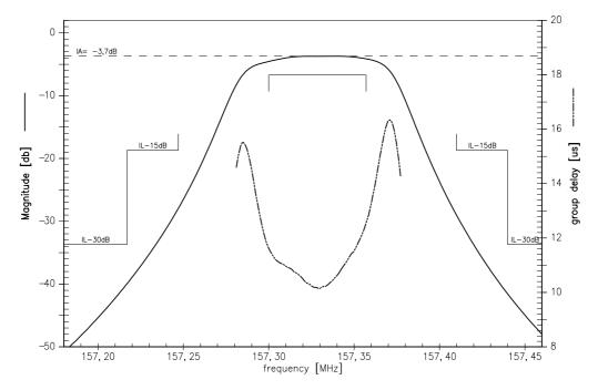
Transfer function wide band (measured unbalanced / unbalanced)
