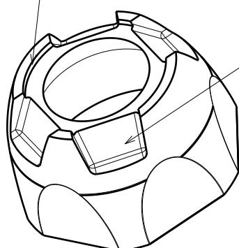
Recesses for solder pads/ screws
