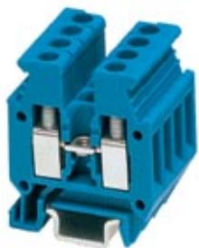
Feed-through terminal block, Connection method: Screw connection, Cross section: 0.2 mm<sup>2</sup> - 4 mm<sup>2</sup>, AWG: 24 - 12, Width: 5.2 mm, Color: blue, Mounting type: NS 15
