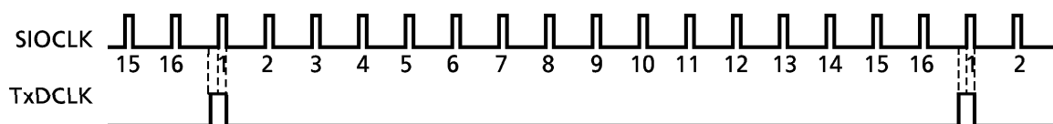
Figure 3.10 (12) Transmission Clock Generation
